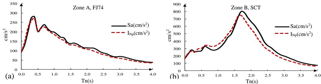
Figure 5. Uniform hazard spectra (250-year return period) for: (a) FJ74 (firm ground) and (b) for SCT (soft soil).
