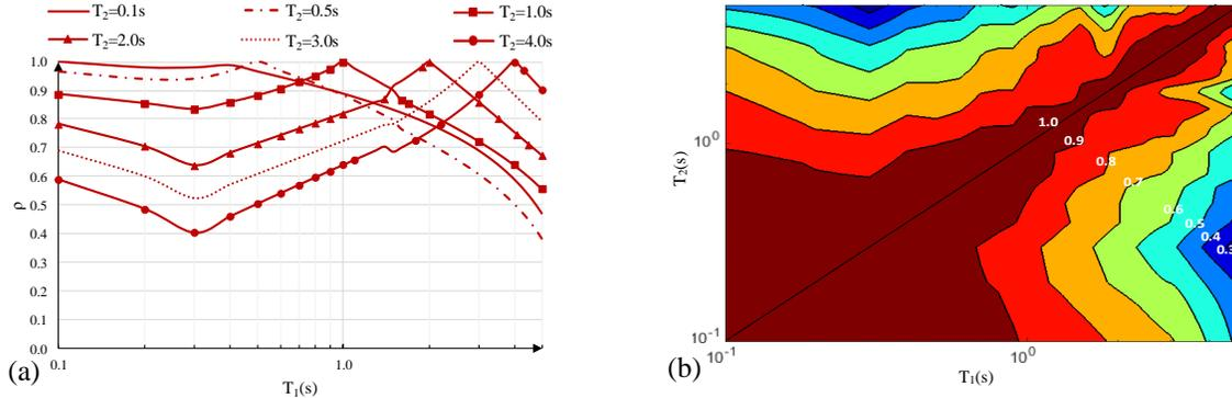
Figure 3. (a) Correlation coefficients versus  $T_1$ , for several  $T_2$  values and (b) Contours of correlation coefficients versus  $T_1$  and  $T_2$ , using equation 1.
