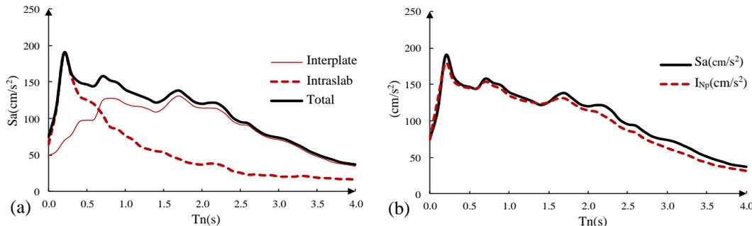
Figure 4. (a)  $Sa(T_1)$  uniform hazard spectra for CU station (interplate and intraslab events) and (b)  $Sa(T_1)$  and  $I_{Np}$  uniform hazard spectra for CU station.
